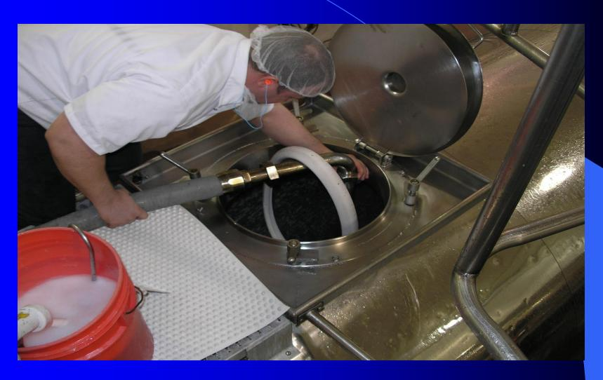
Using soap, water and a brush, thoroughly hand clean the manhole gasket.
