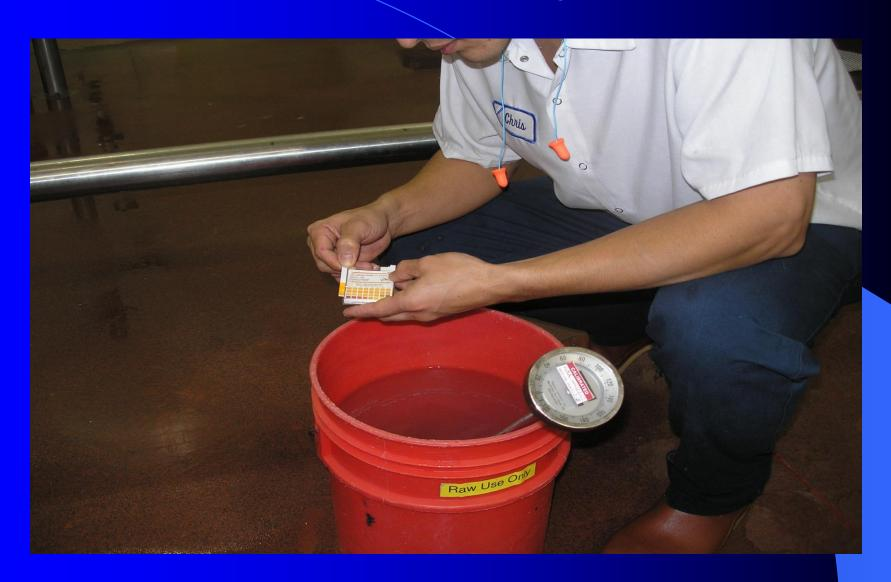
Insert the properly sanitized thermometer into the milk and take a reading. The temperature of the milk must not exceed 45 degrees Fahrenheit. Note: Your Plant may require that milk be colder than 45 degrees.
